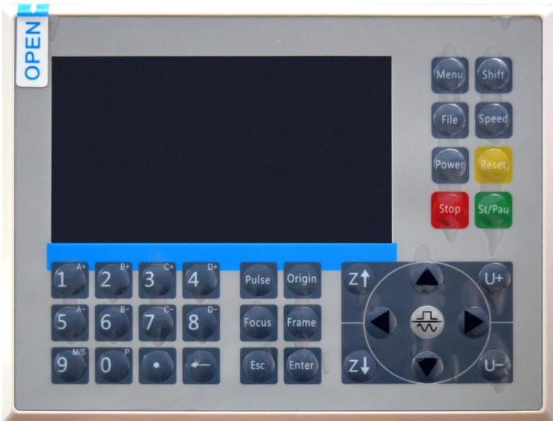
To load a design from a FAT16 or FAT32 formatted flash drive or external hard drive, press MENU, select "File", then "Udisk+", and then "Copy to Memory". Select the design in the File menu, and then select Run. Various parameters can be adjusted using the console's menus and submenus, including setting multiple origins to engrave a design on a material four times in a single session.
