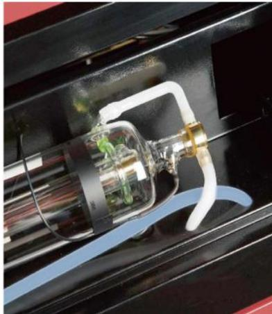
You'll need to place a piece of tape at each stage of the laser path, marking it to confirm that the platform remains properly aligned. If not, you will use the bracket of the laser tube or the screws on the back of the misaligned mirror to correct the problem. Once the supplied tapes run out, we recommend using masked tapes as it is easy to manage and use.
