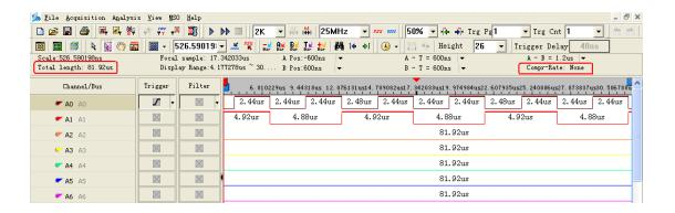
Figure 4-26 Ex: Acquisition without compression – 81.92 us acquisition
