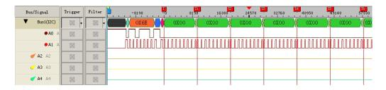
Figure 4-41 Protocol Analyzer Trigger Mark
