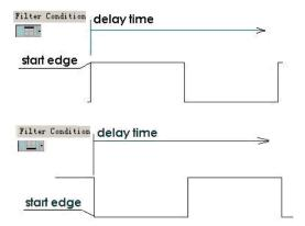
Figure 4-29 Signal Filter / Delay Start Point - Start Edge
