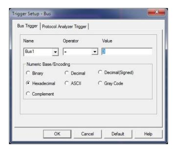
Figure 4-36 Bus Trigger Setup dialog box
