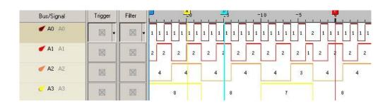
Figure 4-74 Noise filter example / Before applying 5 clock filter
