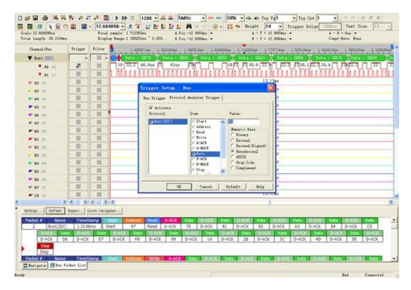
Figure 4-39 Protocol Decoder Trigger example
