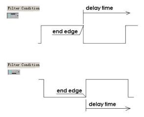
Figure 4-30 Signal Filter / Delay Start Point – End Edge
