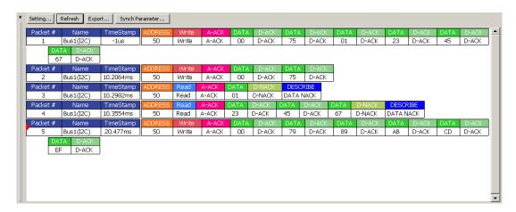
Figure 4-91 Packet List example showing an I2C protocol
