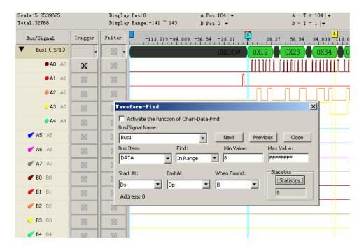
Figure 4-60 Find example: B-bar seen at start of SPI data 0X12
