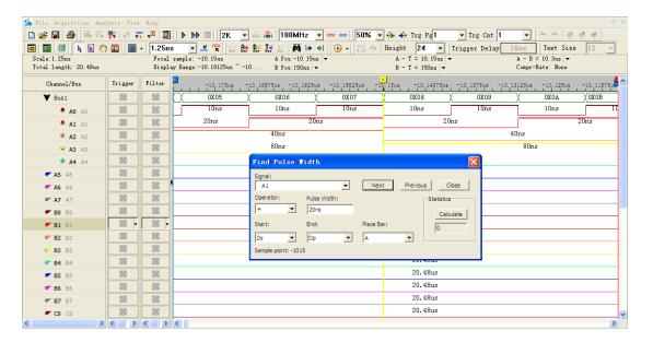
Figure 4-64 Find Pulse Width example
