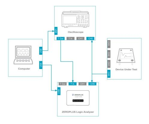
Figure 4-50 Connection diagram with LAP-C as Slave
