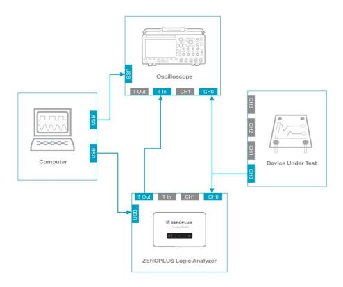
Figure 4-49 Connection diagram with LAP-C as Master
