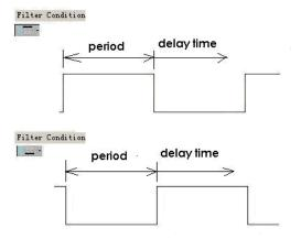
Figure 4-31 Signal Filter / Delay Start Point - Period + Delay
