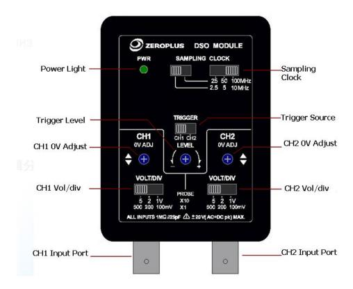
Figure 4-107 DSO Module Setting Panel
