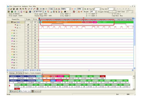
Figure 4-95 Synchronize Navigation example in red frames
